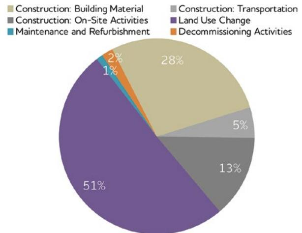
FIGURE 37: CONAWAPA GENERATION PROJECT LCA RESULTS – GHG EMISSIONS PER PRIMARY ACTIVITY [PEMBINA INSTITUTE, 2013]
