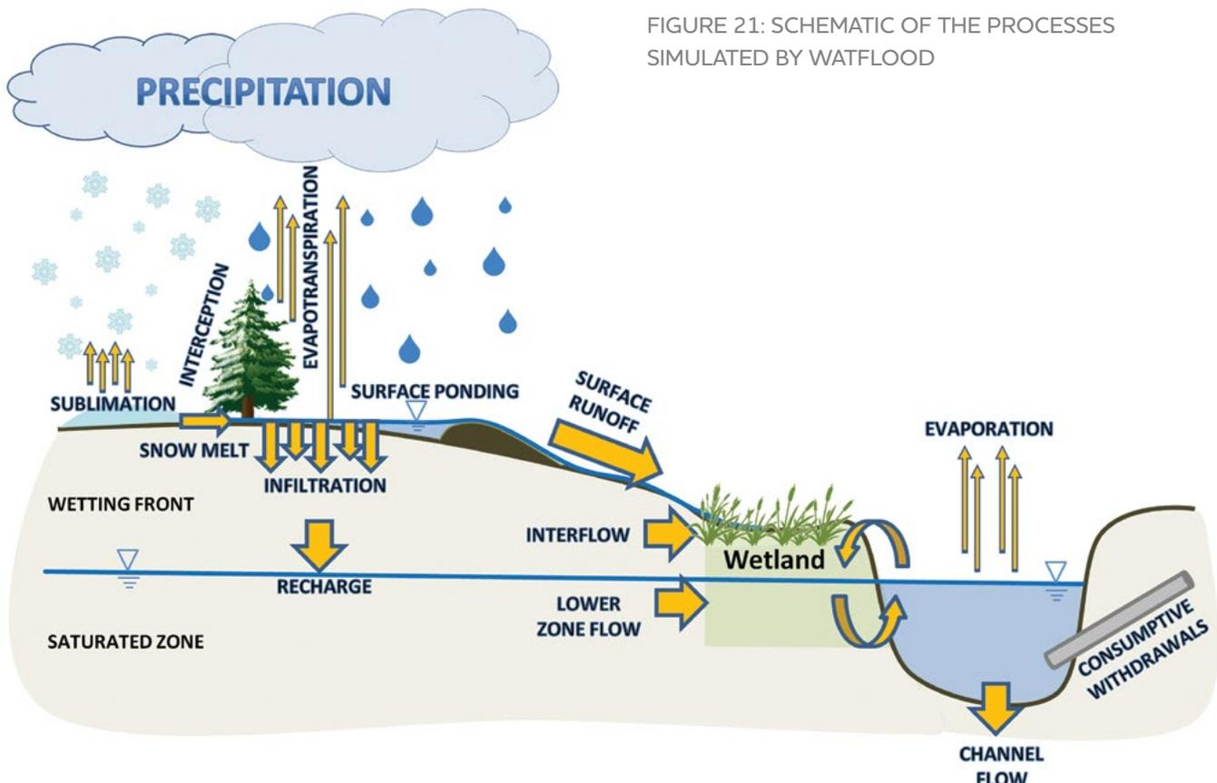
FIGURE 21: SCHEMATIC OF THE PROCESSES SIMULATED BY WATFLOOD
