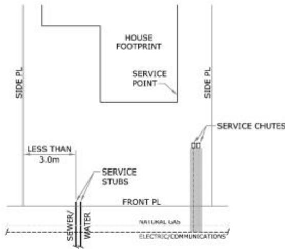
**FIGURE 28 - ALTERNATE SERVICE STUB LOCATION
