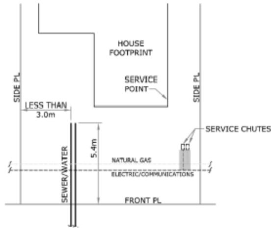
**FIGURE 24 - ALTERNATE SERVICE STUB LOCATION
