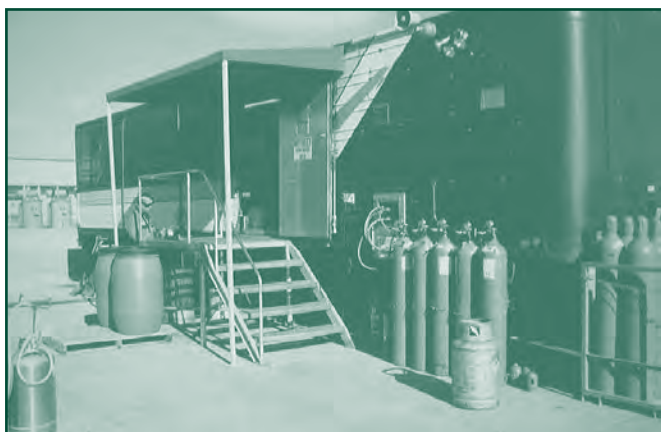
Manitoba Hydro's mobile PCBX decontamination unit, purchased in 1985, was the first of its kind in Canada. In addition to the mobile facility, Manitoba has PCB storage and laboratory facilities.
