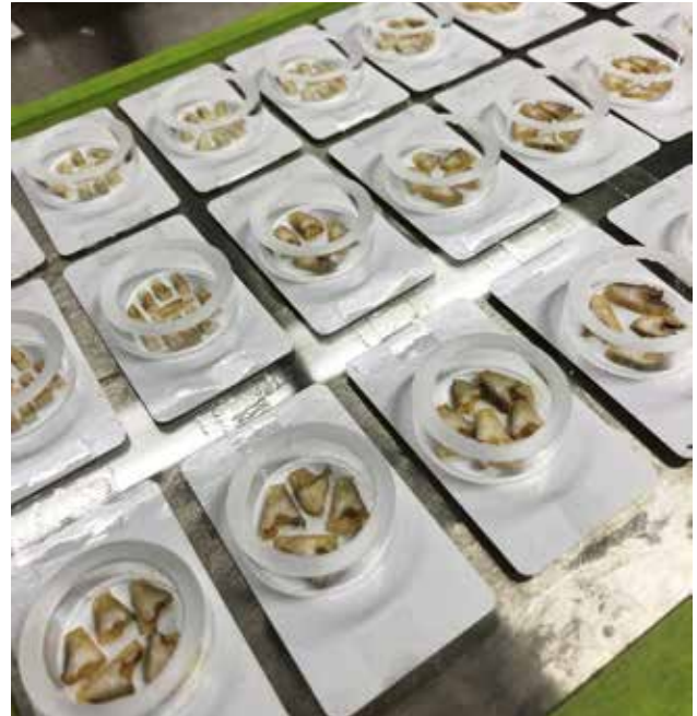
Lake Sturgeon fin ray sections being prepared for laser ablation analysis
