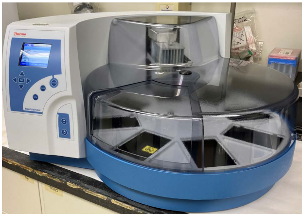
Robotic nucleic acid extractor used to prepare DNA from Lake Sturgeon tissue samples infected with a novel herpesvirus
