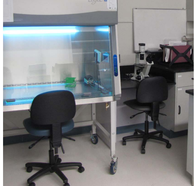
Biological safety cabinet and microscope used to work with and visualize novel Lake Sturgeon viruses
