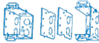
REMOVE ONE SIDE FROM EACH BOX
