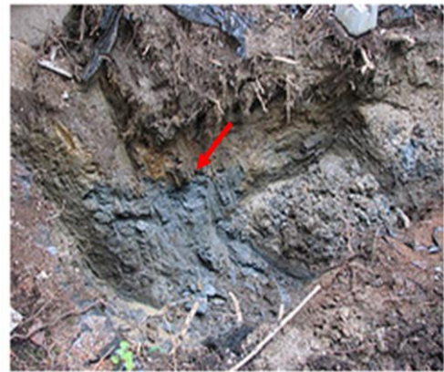
Photo 2: Black PHC, PAH, and/or PCB soil staining
