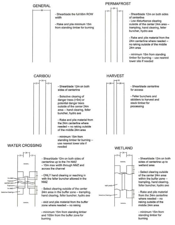
Note: Riparian Buffers for Water Crossings and Wetlands are a minimum of 30m but increase in size based on slope of land entering waterway. (See Riparian Buffer Table in CEnvPP)
