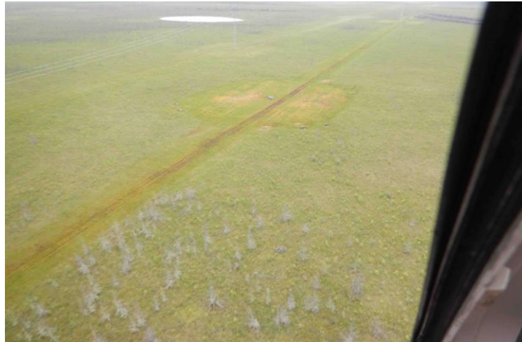
Photograph 4-3b. Rutting in wetlands from construction activities.
