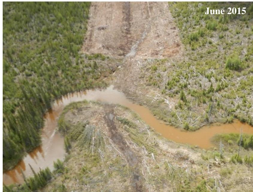
Photo 4. N1-Aqua-133 (unnamed tributary of South Moswakot River). Channel runs within the riparian buffer zone in the RoW, prone to erosion, June 2015.
