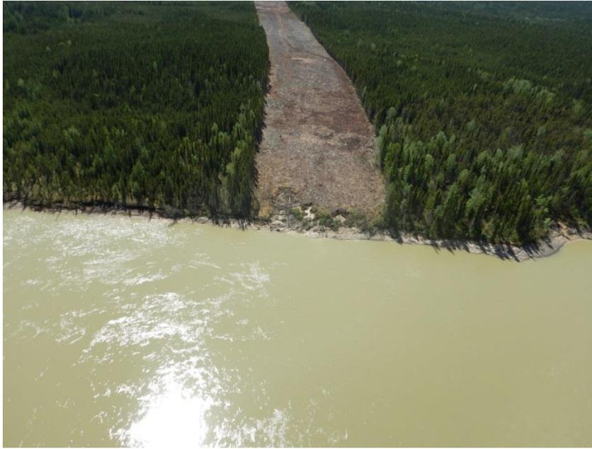
Photo 7. N1-Aqua-173 (Burntwood River). Erosion in RBZ and slumping of southern bank (segment N1), June 2015.
