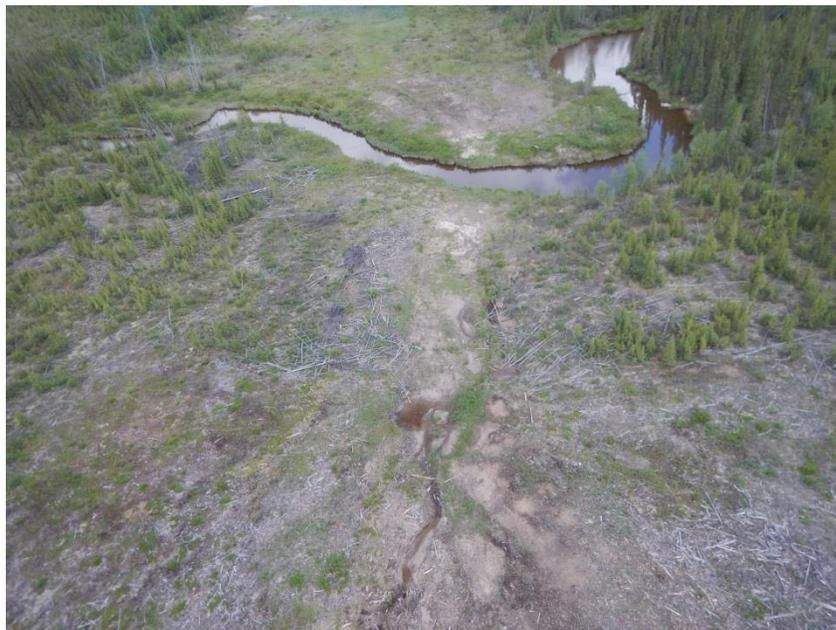
Photo 6. N1-Aqua-133 (unnamed tributary of South Moswakot River). Channel runs within the riparian buffer zone in the RoW, prone to erosion, June 2017.
