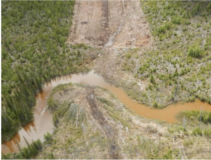
Photo 5. N1-Aqua-133 (unnamed tributary of South Moswakot River). Channel runs within the riparian buffer zone in the RoW, prone to erosion, June 2015.
