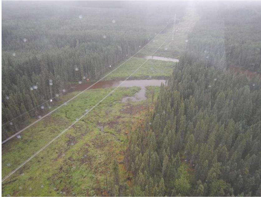
Photo 25. N3-Aqua-103 (Mitishto River). Shrubs and forbes becoming established on the banks through erosion control matting, June 2017. No erosion was detected.
