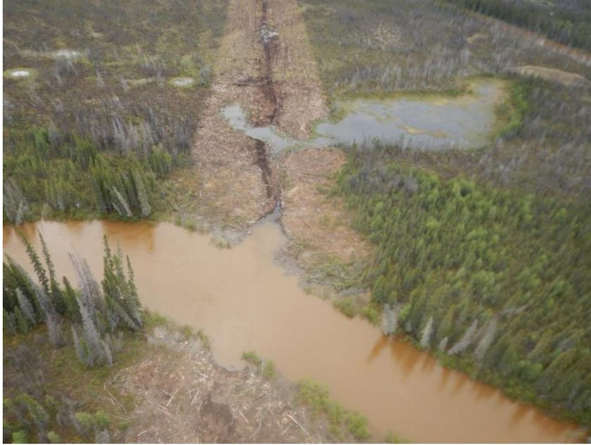
Photo 3. N1-Aqua-129 (Limestone River). Channel within RoW is subject to erosion, June 2015.
