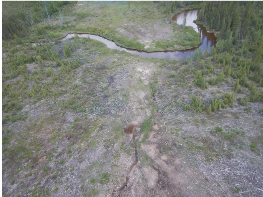
Photo 5. N1-Aqua-133 (unnamed tributary of South Moswakot River). Channel runs within the riparian buffer zone in the RoW, prone to erosion, June 2017.
