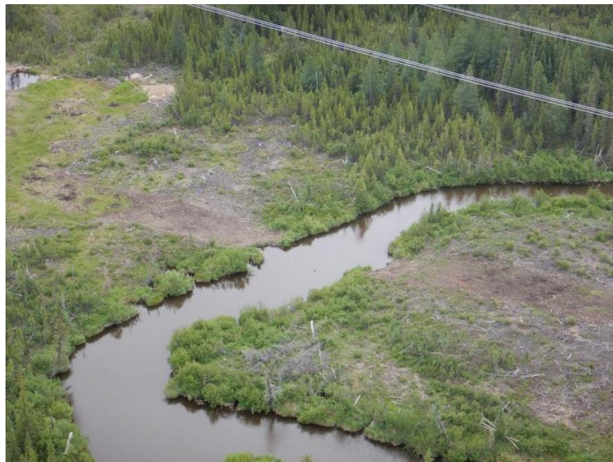
Photo 7. N1-Aqua-131 (North Moskwakot River). Presence of bare ground through the RoW at the centerline trail crossing is susceptible to erosion. regrowth occurring but suggest implementing ESC measures due to important fish habitat, June 2018.
