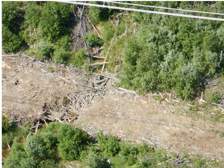
Photo 21. N1-Aqua-169 (unnamed tributary of Odei River), June 2018. Temporary crossing has remained in place since first observed in 2015. Marginal fish habitat therefore removal should be considered.
