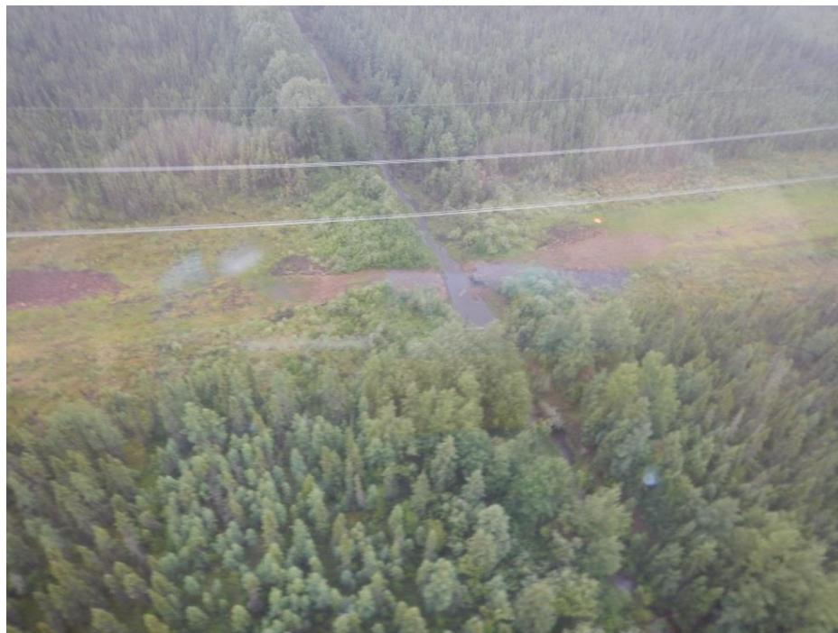
Photo 25. N3-Aqua-107 (unnamed tributary of the Mitishto River). Steep bank on the centerline trail with exposed soil, June 2017.
