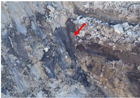
Photo 1: Grey-black PHC, PAH, and/or PCB soil staining
