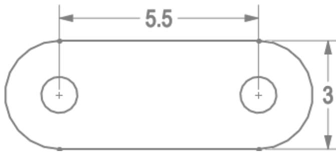
Figure A-3. Tower base dimensions (m) with 1 m safety buffers for H-frame tower.
