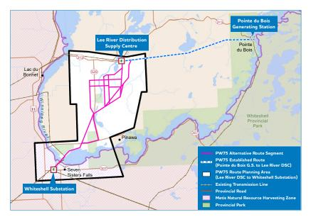
Map of alternative route segments for the new 115-kV transmission line from Pointe du Bois Generating Station to Whiteshell Substation. View enlarged map at **hydro.mb.ca/prep**. Feedback received in our engagement will help determine the preferred route.
