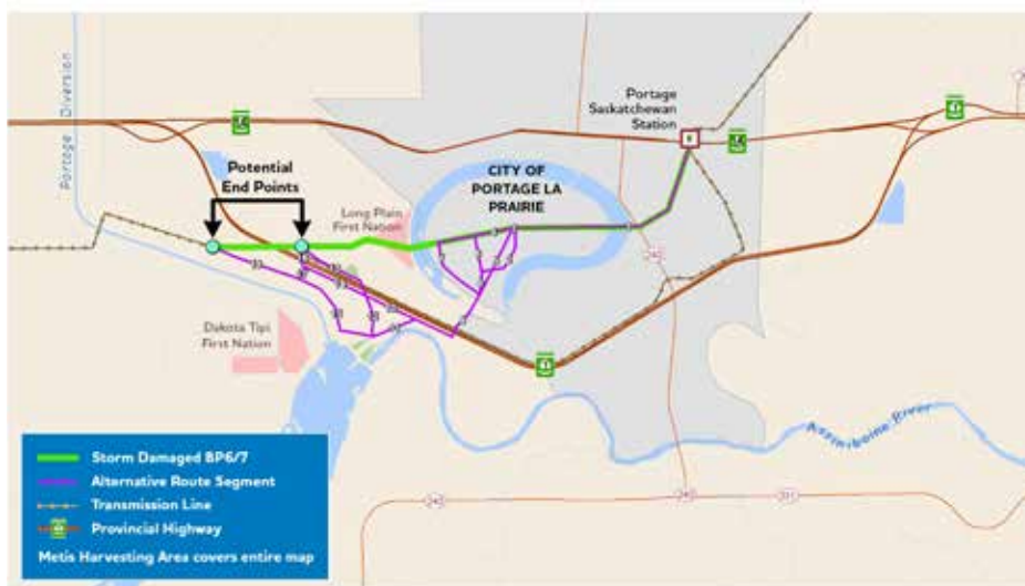
Map of the Portage la Prairie area showing sections of BP6/BP7 that need to be rebuilt and rerouted.
