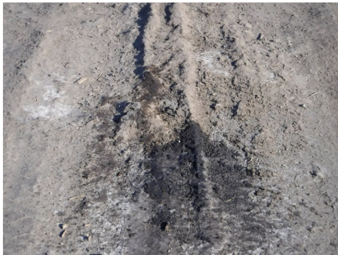
Photo 2: PHC (oil) staining clay soil
