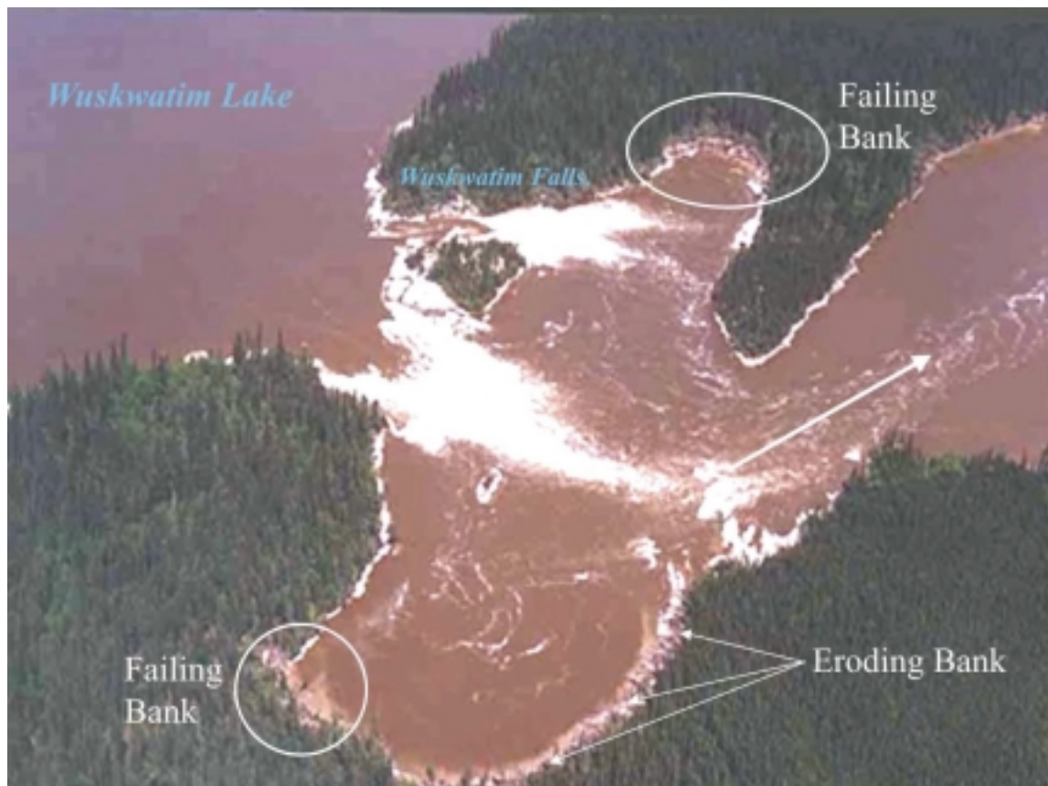
Figure 6.3-24. Oblique aerial photograph showing the location of failing and eroding banks below Wuskwatim Falls. View looking towards the north.
