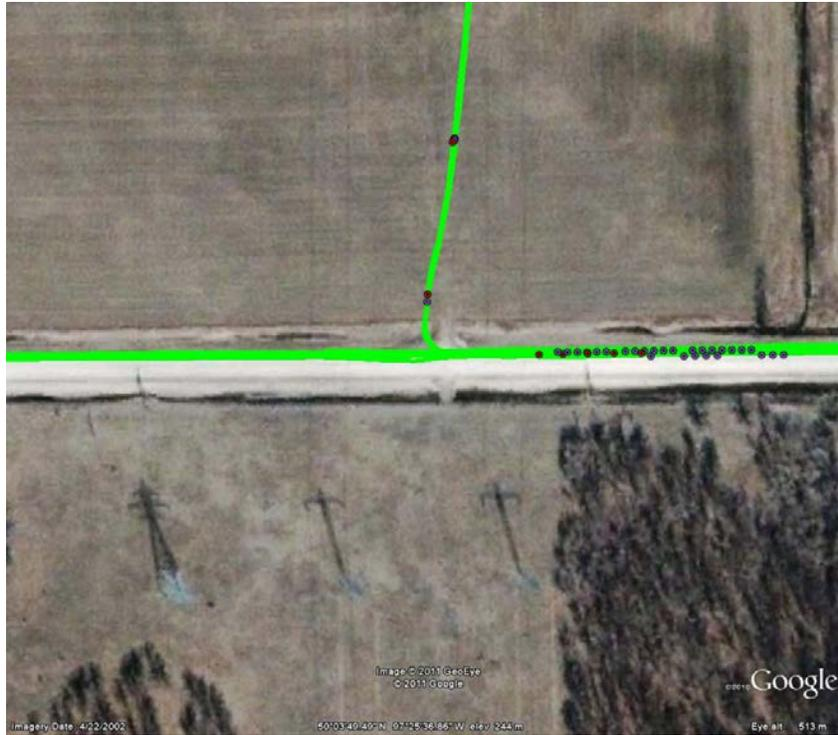
Figure 20 – Geo-Located Cycle Slips (red: 24 Jan, purple: 25 Jan)
