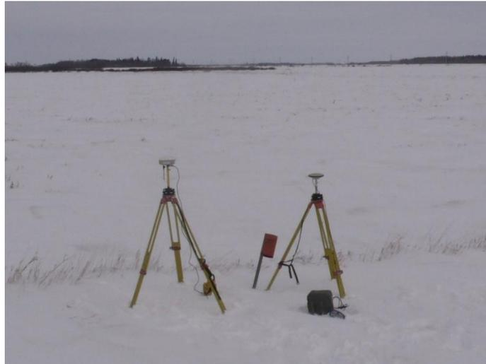
**Figure 2 – Deployment of GNSS base stations on 24 January 2011. Novatel V3 receiver utilizes right tripod equipped with a Novatel 702-GG GPS+GLONASS L1+L2 antenna. Trimble R8 base unit occupies left tripod, with integrated receiver + antenna + radio module. Radio antenna is the black vertical bipole antenna visible under the R8 receiver body.**
