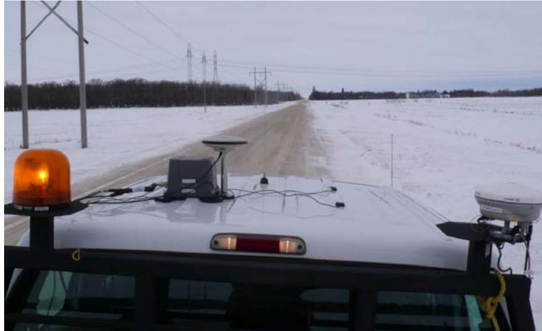
**Figure 4 – Mobile GNSS, Inertial, and RF equipment elements mounted on roof of test vehicle. Trimble R8 rover unit at bottom right, high sensitivity GPS antennas on roof at right, Novatel 702 GG dome antenna centre left directly adjacent to LCI IMU (grey box) at centre left.**
