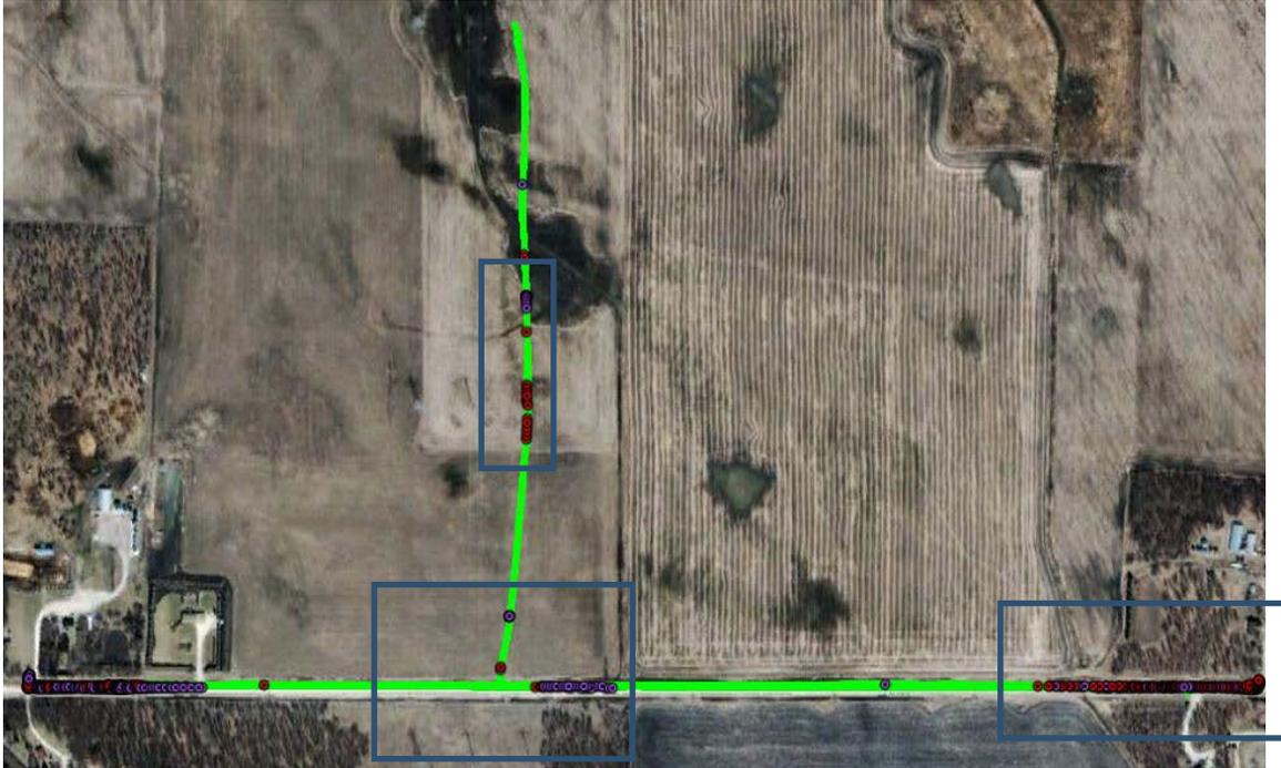
**Figure 18 – Geo-Located Cycle Slips (red: 24 Jan, purple: 25 Jan), blue rectangles indicate Figure 19, Figure 20 and Figure 21**
