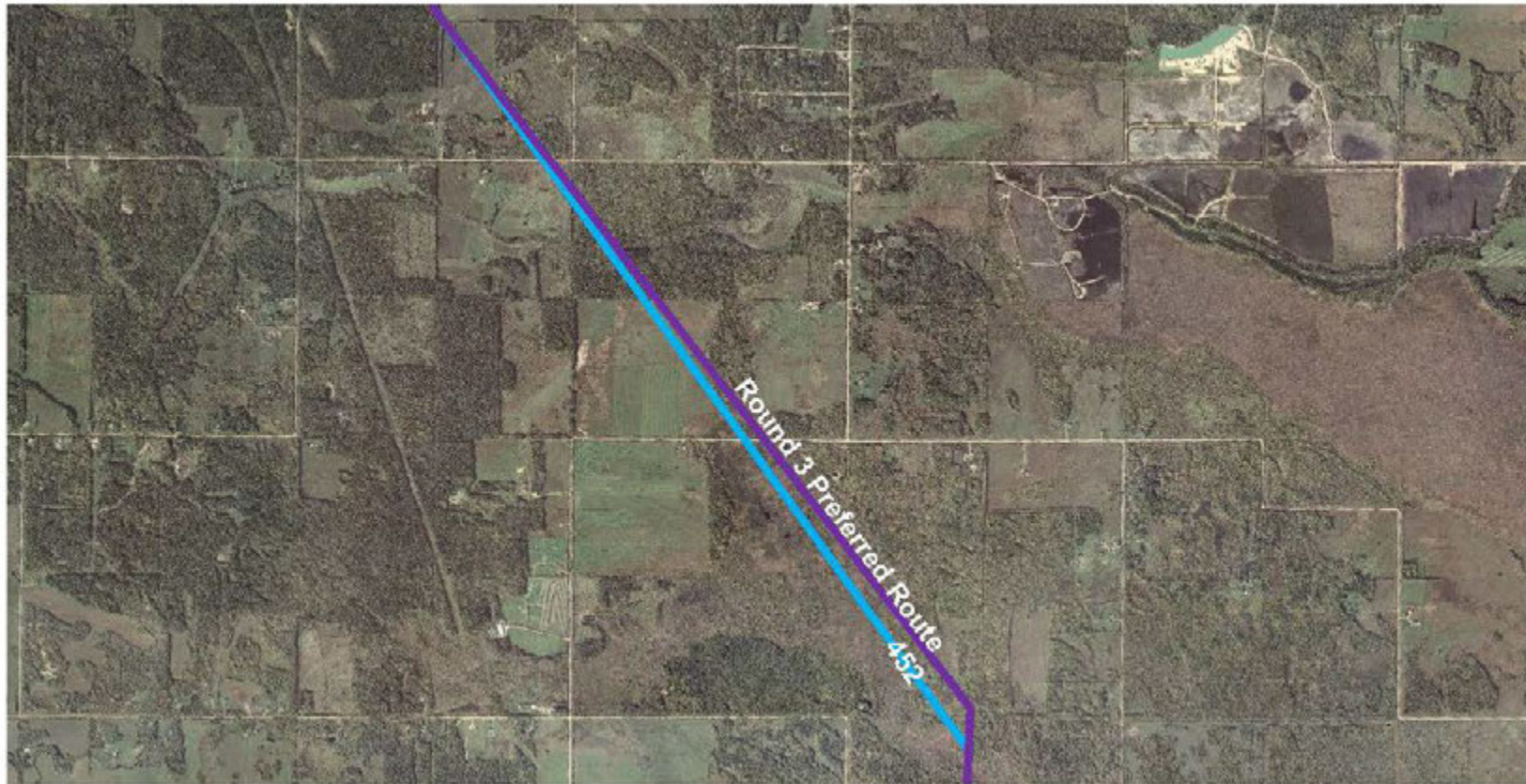
Figure 5-26 Segment 452 (blue line) was Created to Equalize Distances between Houses North and South on the Line
