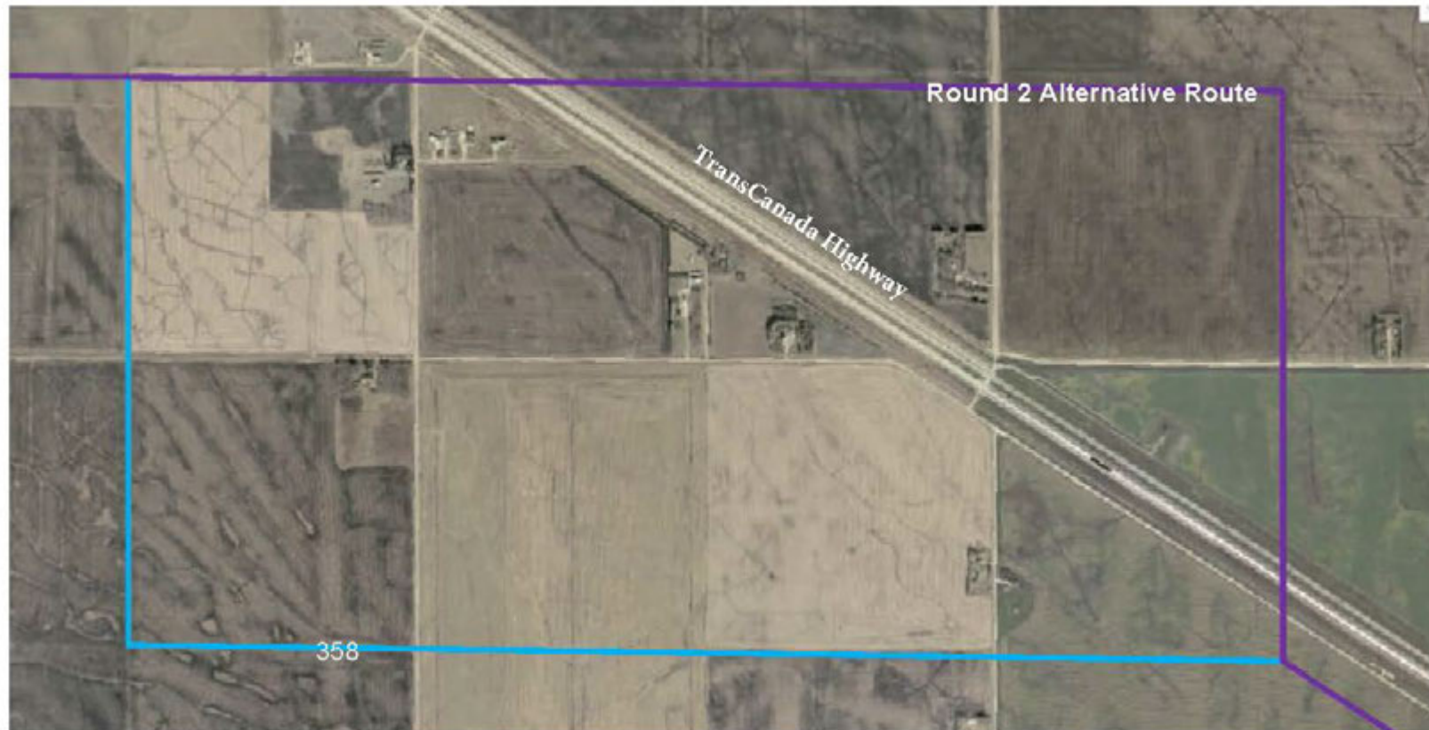
Figure 5-10 Segment 358 (blue line) was Created to Avoid two Homes and two Crossings of the TransCanada Highway
