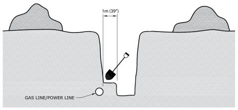
Dig a trench or bell hole 1 metre from the line location, parallel to the line, then hand dig laterally to expose the line.
