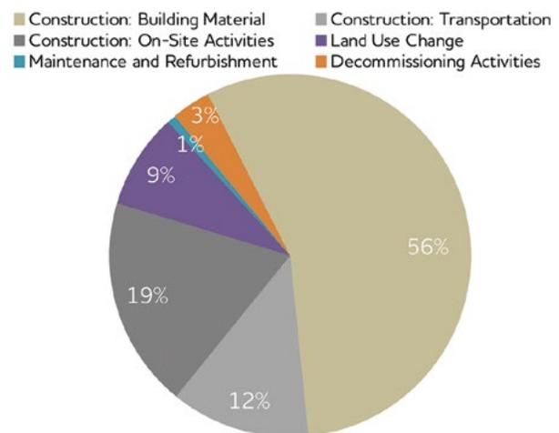
FIGURE 38: NATURAL GAS COMBINED CYCLE PLANT: LITERATURE SURVEY OF LCAs – GHG EMISSIONS PER PRIMARY ACTIVITY [PEMBINA INSTITUTE, 2013]
