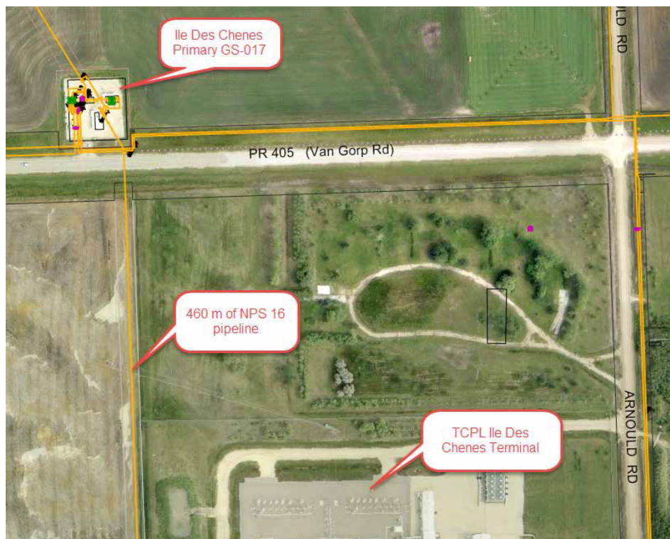
FIGURE 15 – 460 M OF NPS 16 PIPELINE FROM TCPL TO GS-017
