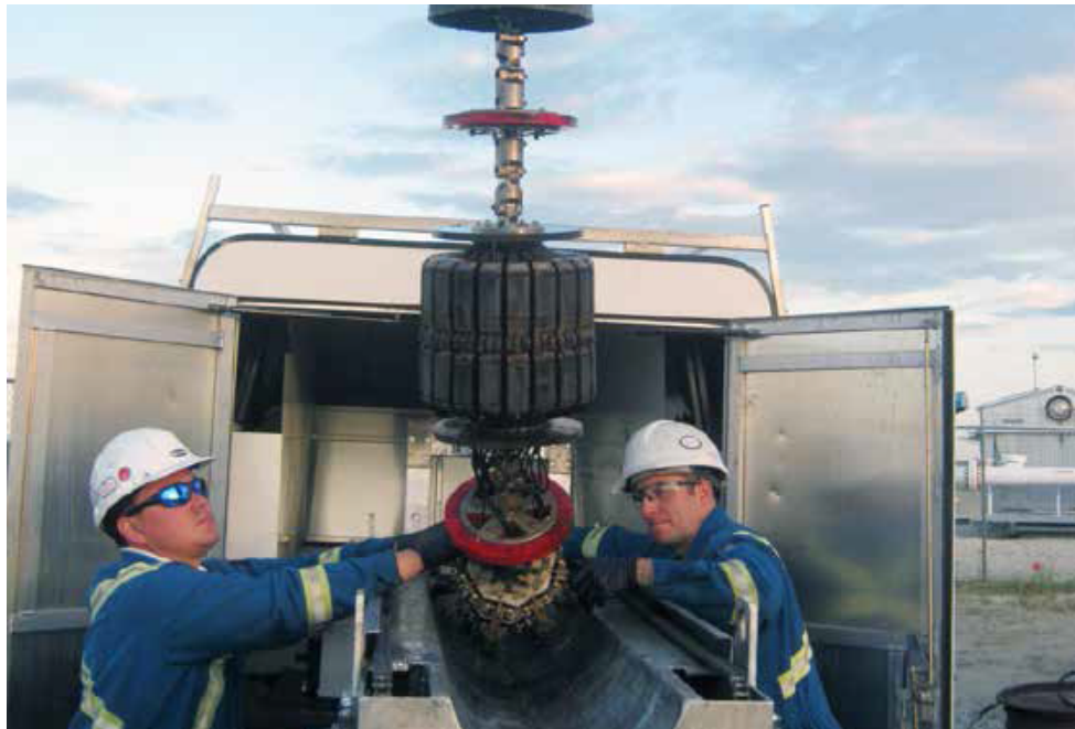
FIGURE 34 – LOADING OF IN-LINE INSPECTION TOOL AFTER PIPELINE INSPECTION
