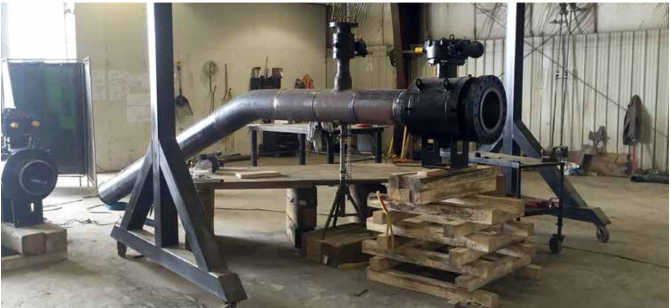
FIGURE 6 – PIG LAUNCHER FABRICATION
