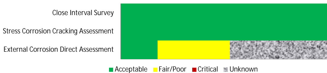
Figure 13: Percentage of unassessed asset condition of transmission pipelines based on findings from condition monitoring programs specific to degradation “soccer field”. 100% represents that sample size of pipeline by km for each assessment methodology.
