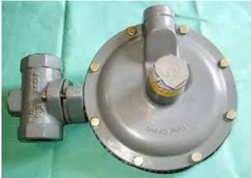
Figure 13: Typical residential regulator
