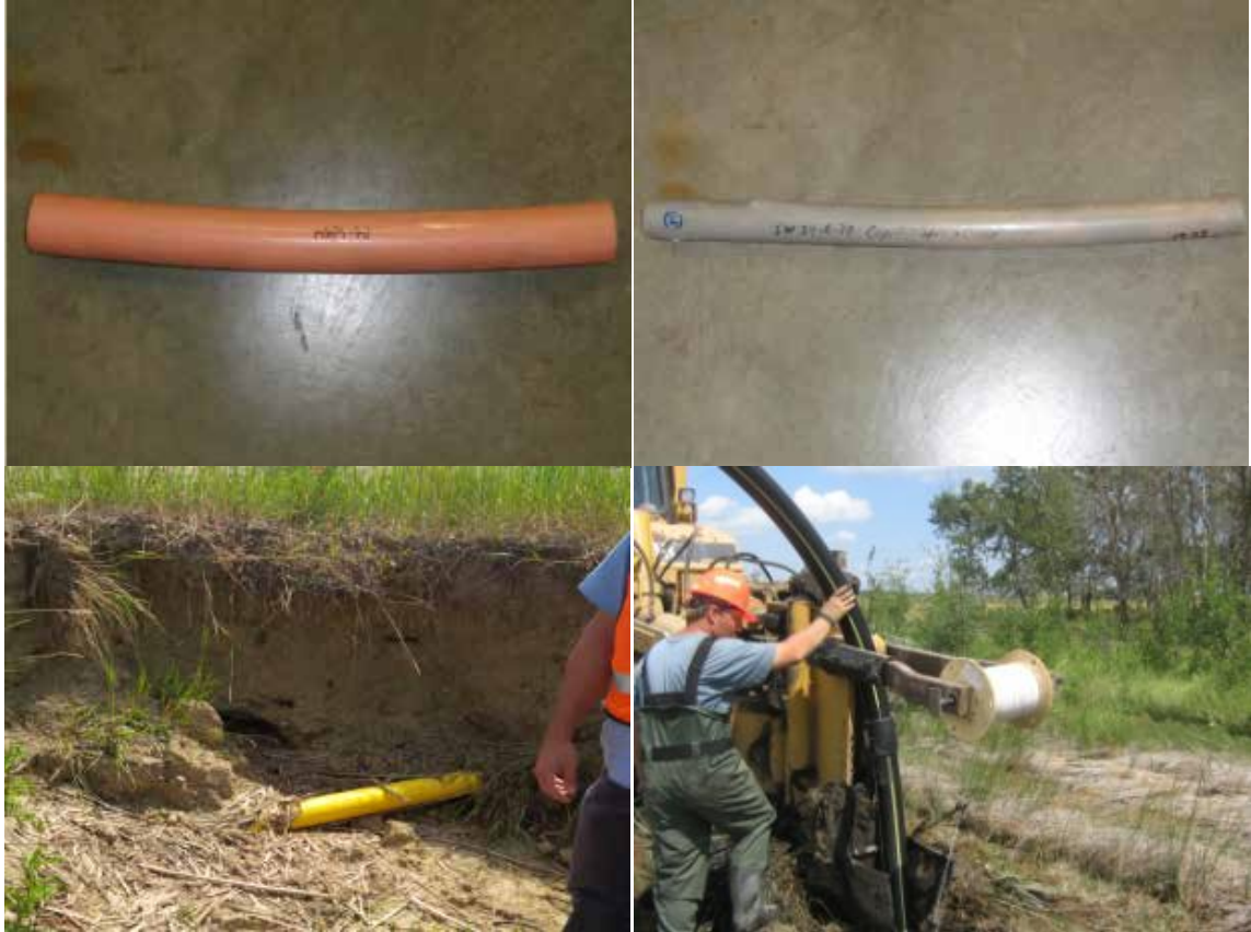
Figure 4: Various types plastic pipelines: PE 2306 Aldyl-A (top left), Aldyl-A pipe with grey pigment due to reaction with soil (top right), PE 2406, commonly PE (bottom left) and PE-100 a.k.a. PE 4710, commonly HDPE, (bottom right).
