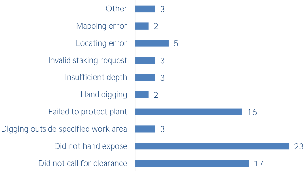
Below Grade Natural Gas Damages by Cause 2016-17
